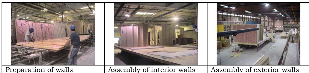
Figure 4.15 Wall installation phase of MH production
